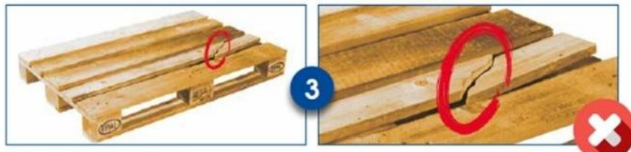
3 A board is damaged
