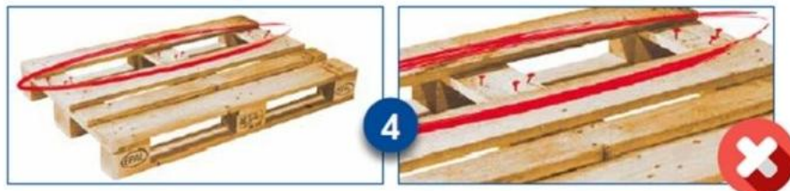
4 A board is missing
