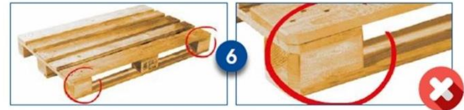
The EPAL mark is missing on the side blocks (if the pallet was produced after August 1, 2013); The EUR mark on the right and the EPAL mark on the left are missing (if the pallet was produced before August 1, 2013)
