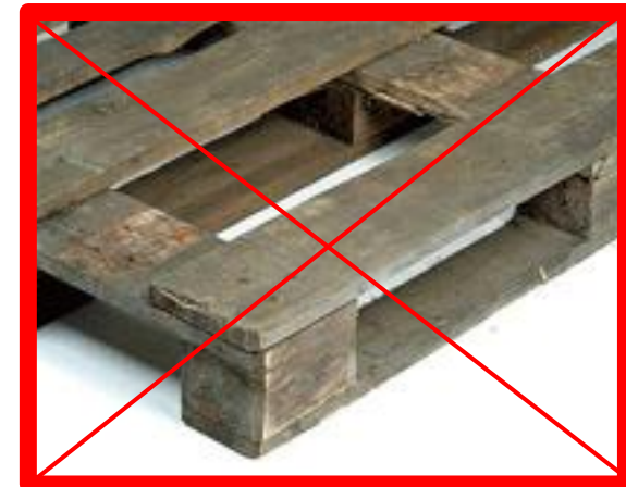
Missing top board
