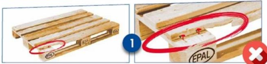
1 A board is damaged and exposes the nails
