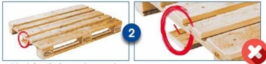
2 A block is missing or damaged
