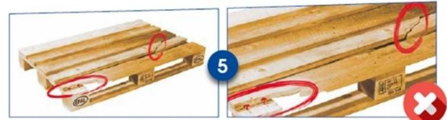
5 More than 2 boards are damaged
